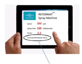
A Servo performance menu is available to display the *actual* displacement of the servo compared to the *theoretical*.
